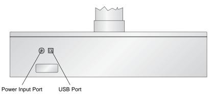
The **Power port** connects to a 12v 5 amp power converter. The **USB port** connects to a standard 6' USB cable. Plug the other end directly into a USB port on the back of your computer.
